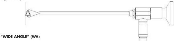
"Wide angle" telescopes provide a bigger field of view.
